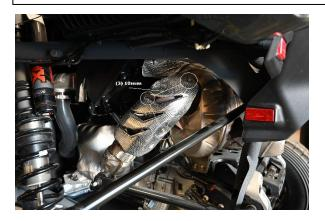
2. To remove the factory muffler, you'll need to remove the heatshield covering the head pipe which is held on by 3 10mm bolts. Then, remove the 4 springs holding on the exhaust head pipe and the 3 bolts holding the muffler to the frame of the vehicle located beneath the muffler assembly along with the 1 bolt located behind the muffler assy.
