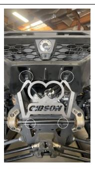
4. Finally, install muffler assy #A by fishing it through the passenger side wheel well. Be cautious and patient when fishing it into place as it is a bit of a tight fit. When finished, install tips #E
